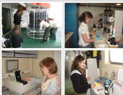
Figure 6. CTD/rosette and instruments employed for the hydrographic characterization.
